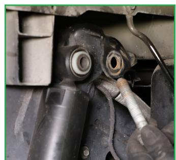
9. Remove the nut and bolt from the bottom shock mount. (Figure 29)
